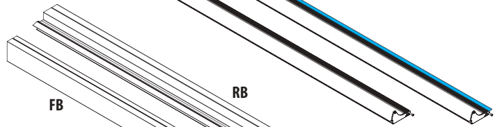
Left gutter beam & right gutter beam (lateral beams) (RG, LG)
